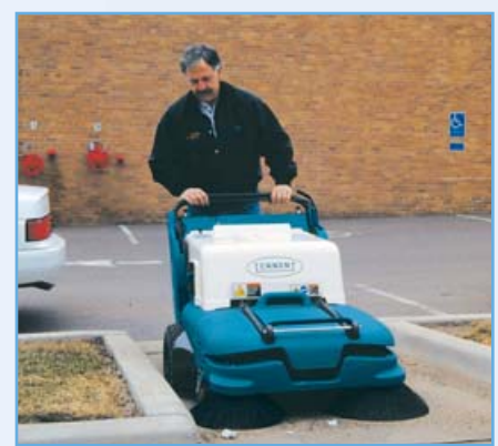
An optional outdoor package comes with wide pneumatic tires and larger front casters.
