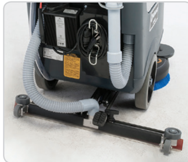
Center-pivot squeegee system employs a gas spring for maximum blade pressure to ensure complete dirty solution pickup in both forward and reverse.
