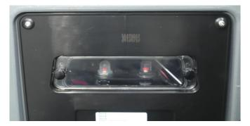
When the overload reset switch triggers a power trip, please determine the cause of the power trip and let the motor cool down, and then manually press the overload reset switch button.
