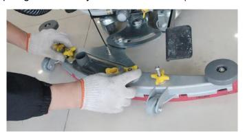
2. Unscrew the two yellow nuts on the outside and turn them to the top. Turn the squeegee over and take out the blade (as shown in the figure below).
