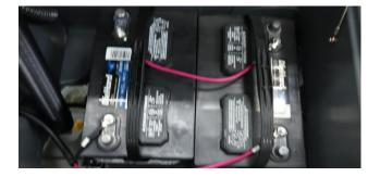
Maintenance every month: check distilled water levels in battery cells.
