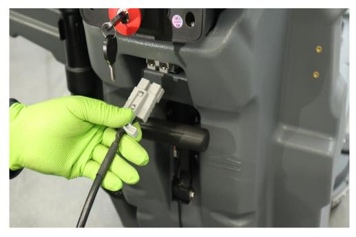
Note: During the charging of the charger, please do not unplug the DC cable of the charger from the socket on the machine. In order to avoid arc discharge. If charging must be suspended during charging, please unplug the AC power cord first.
