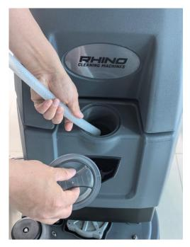
For scrubbing method: use warm water (maximum 60°C). Pour the recommended detergent into the solution tank for mixing.
