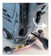
and turn on the brush plate switch (as shown in the picture below).
