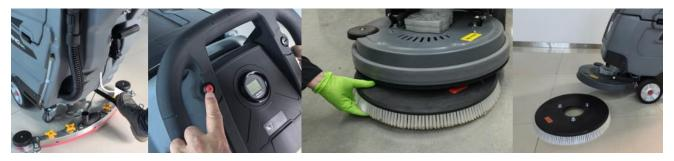
4. Clean the squeegee blade (as shown below). Place the squeegee in a raised position to prevent damage to the blade.
