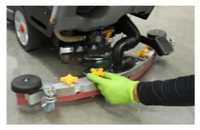
4. Connect the suction pipe to the squeegee assembly (as shown in the figure below).
