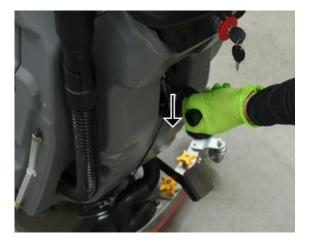
• Manually adjust the valve, adjust the amount of water output. After adjusting it to the appropriate position, push the machine to start cleaning (as shown in the picture below).
