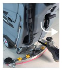
3. Place the brush plate in the center of the brush plate cover, hold the brush plate upward with both hands in balance, and put one pin on the brush plate into the brush buckle installation hole through the observation port, and shake it from side to side, so that the other two pins also enter the hole of the brush buckle. When the brush plate is balanced, then immediately forcefully rotate counterclockwise, and snap into the brush buckle by inertia (as shown in the picture below).
