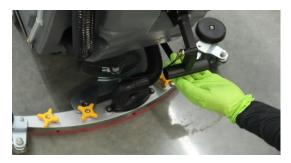
3. Install the squeegee assembly on the squeegee mounting bracket (as shown in the figure below). Be sure to put the tightening knob completely into the slot before tightening the knob.
