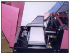
The panel filter system captures fine dust and drops it directly into the hopper. This system provides longer dust-free sweeping performance.
